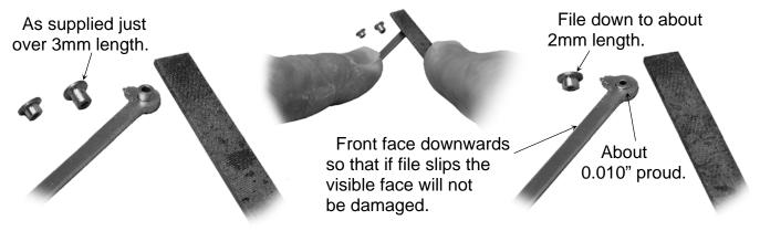
These bearing bushes are not soldered into the rods but locked onto the crankpin with a nut & washer. So it is important that they will revolve freely in the holes in the rods.
