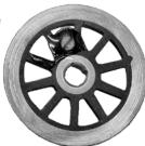
Fit balance weights using a generous application of Araldite. An etched rear rebate should aid positioning just below turned wheel rim.
